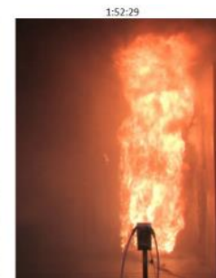
Photos of NMC sprinklered test during fire development on main rack: first sprinkler operation (left) and peak heat release rate (right).
