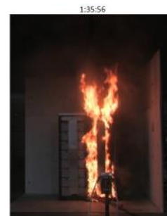
Photos of NMC sprinklered test during fire development on main rack: first sprinkler operation (left) and peak heat release rate (right).
